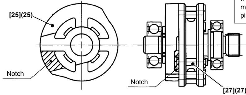
Pay special attention to the position of the Position Detector [25](25). If the Position Detector [25](25) is misaligned, the standby position of the piston is also misaligned. (See page 29.)
