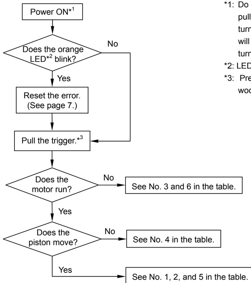
\*1: Do not press the pushing lever and/or pull the trigger during the process of turning the power switch ON. Doing so will prevent the power switch from turning ON.
