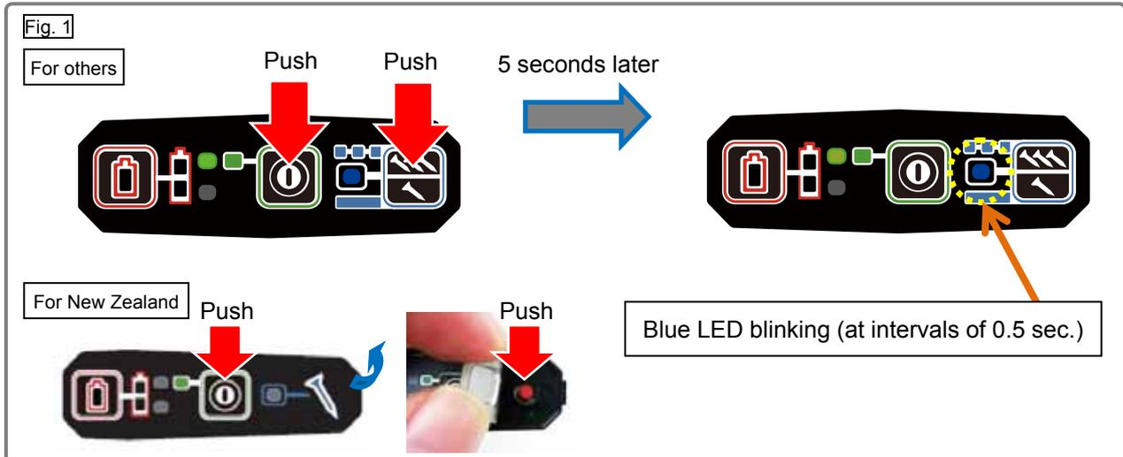
Indication: Indicated by the blue LED on the operation panel blinking (at intervals of 0.5 second).
