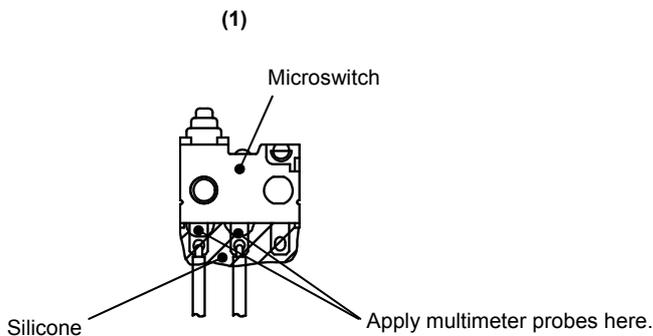
**NOTE: Remove the silicone a little and apply the multimeter probes to the exposed terminal metal.**
